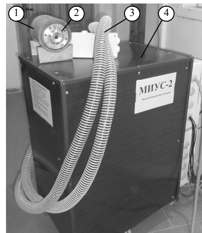
Fig. 3. The laboratory equipment for EMF attraction processes with maximum charging voltage of 2kV and accumulated energy of 2kJ: 1 – pulsed current transformer; 2 – single turn inductor; 3 – cable connection; 4 – pulse generator
