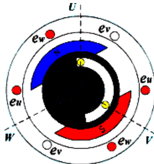
Fig. 2. Valve electric motor
