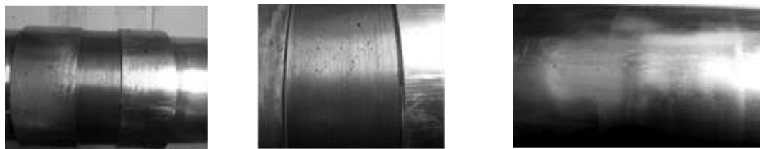
Fig. 7. Striker after operation: wear of the surface
