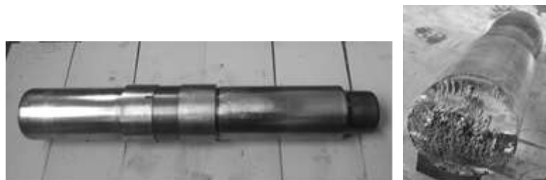
Fig. 3. Hammer striker (general view) and fatigue failure of the hammer striker in the process operation
