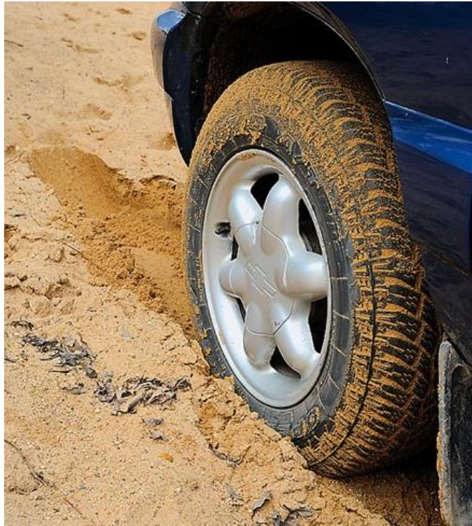
Fig. 75. Elastic wheel on a deformed base
