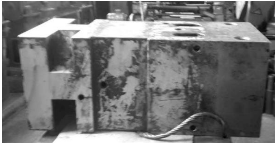
Figure 1.35. Frame hydraulic hammer: A - new; b, c – after use
