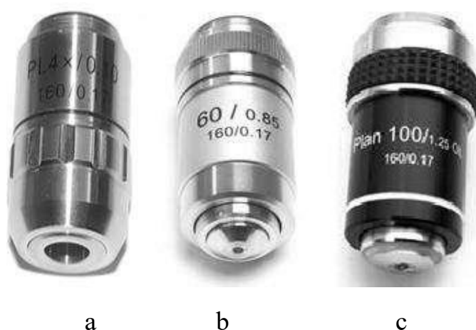
Figure 2.2. Lenses For microscope Altami - MET1 [37]: a – objective lens manufactured by Biomed; planachromat, magnification 4x, numerical aperture 0.10, length of microscope tube, With which lens will work as usual, 160 mm, cover glass thickness 0.17 mm; b – objective lens manufactured by OptiTech; achromatic, magnification 60x, numerical aperture 0.85, length of microscope tube with which the objective lens will work normally, 160 mm, cover glass thickness 0.17 mm; in – objective lens manufactured by OptiTech; plan achromat, magnification 100x, numerical aperture 1.25, length of microscope tube, With which lens will work as usual, 160 mm, cover glass thickness 0.17 mm, oil immersion objective
