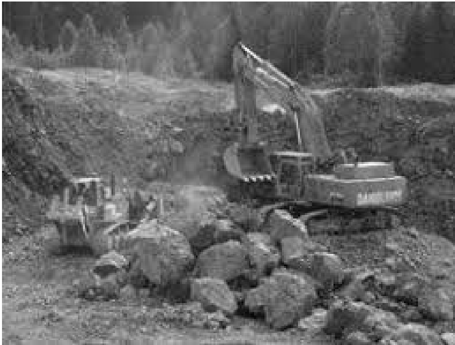
Figure 1.22. Development of rock mass: the average daily capacity of the quarry is 1000 m 3 (750 m 3 in the original); is provided by the simultaneous operation of four hydraulic hammers [4]
