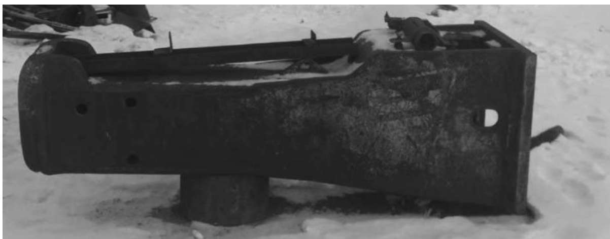
Figure 1.36. Casing (frame) hydraulic hammer after exploitation
