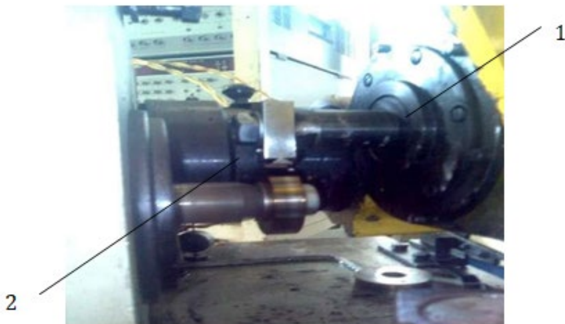
Figure 2.9. External appearance of the friction machine [ 49 ] : 1 - mechanism loading; 2 - subject sample
