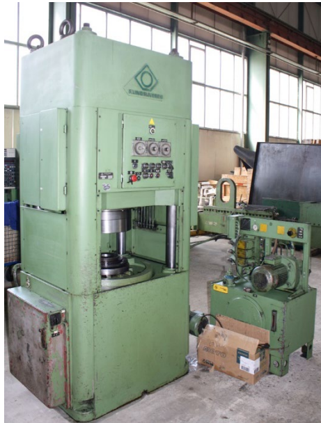
Figure 16.9 – Gear quenching press KLINGELNBERG AH 400 S
