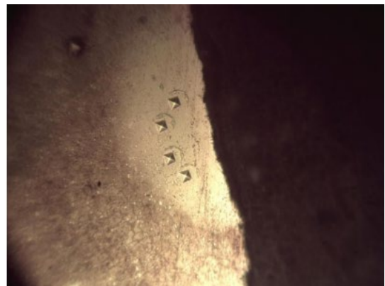
Figure 19.4 – Laser quenching zone (without surface melting)
