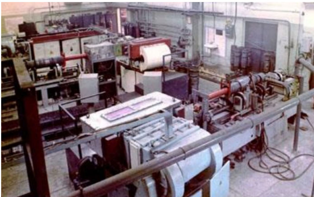
Figure 19.6 – Complex for hardening cylinder liners of diesel engines, laser power 1.5 kW
