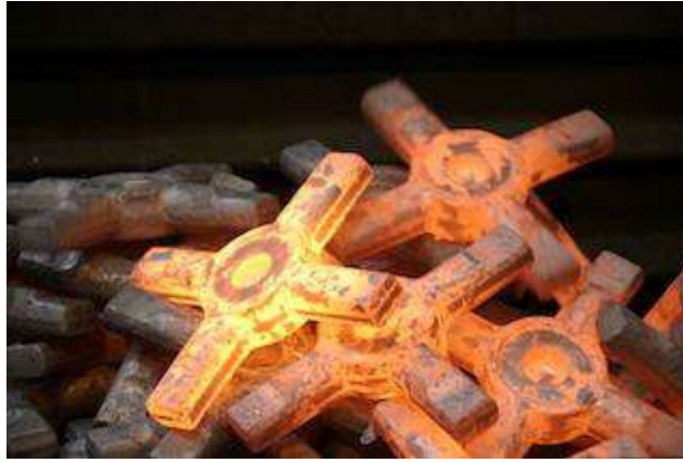
Figure 5. Billets after multiaxial isothermal forging
