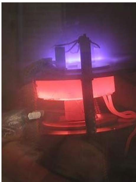
Figure 2. The plasma (violet glow) accelerates the growth of carbon nanotubes in a laboratory PECVD set-up
