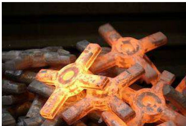
Figure 5. Billets after multi-axial isothermal forging
