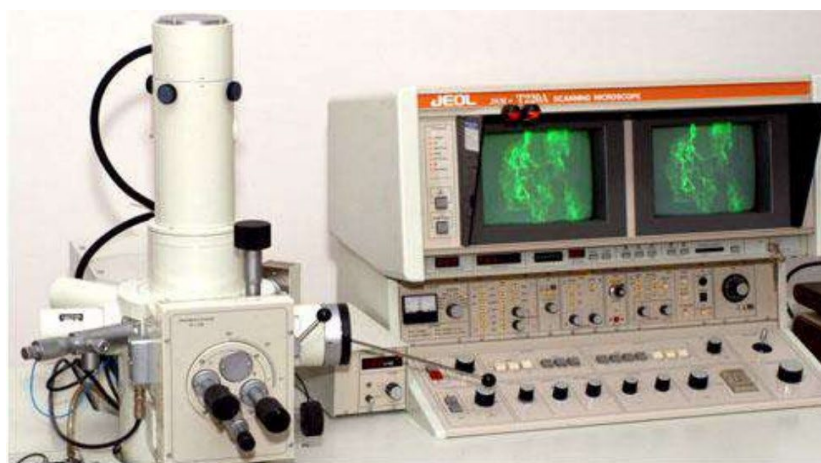
Scanning electron microscope JEOL JSM-T220A
