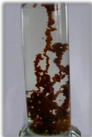
Figure 3. Hydroxide precipitate formed in a test tube during chemical precipitation
