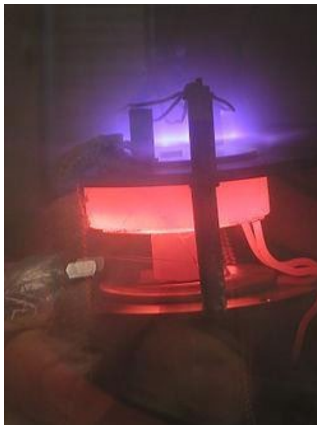
Figure 9. The plasma (violet glow) accelerates the growth of carbon nanotubes in a laboratory PECVD set-up
