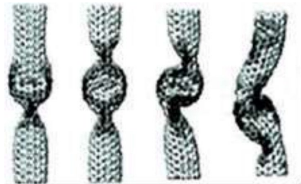
Figure 20. Behaviour of carbon nanotubes under extreme deformation
