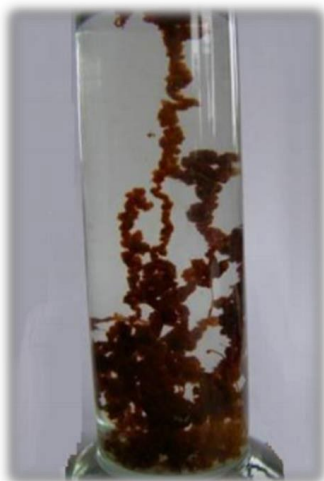
Figure 10. Hydroxide precipitate formed in a test tube during chemical precipitation
