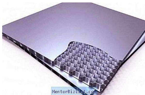
Figure 5. Composite panel with a honeycomb core
