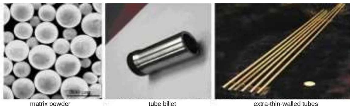
Figure 8. Stages of the production of products from dispersion-strengthened steel
