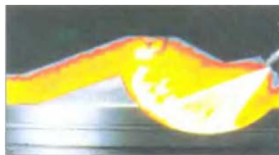
Fig. 12.7. The piston of a direct petrol injection engine has a special shape (combustion process above the piston)
