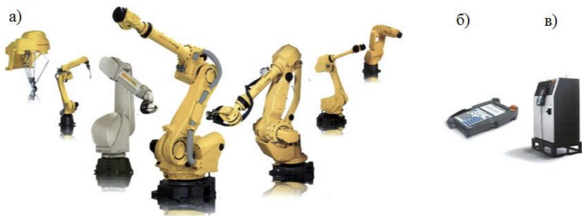
4 - figure. Industrial robots from Fanuc Robotics: a) fragment of the robot model range; b) intelligent portable control panel; c) system controller
