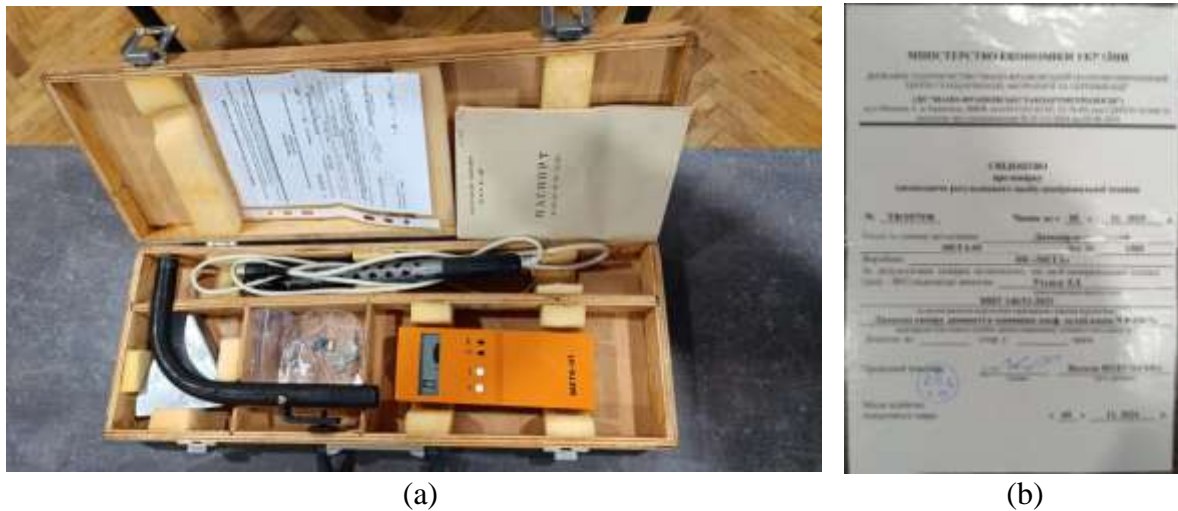
Figure 2 – Opacimeter META-01 for the mobile test bench (a) and its instrument verification document (b)
