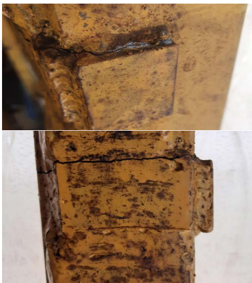
Fig. 2. Damage in the form of cracks in the head of the LIEBHERR 185HC tower crane in Kyiv
