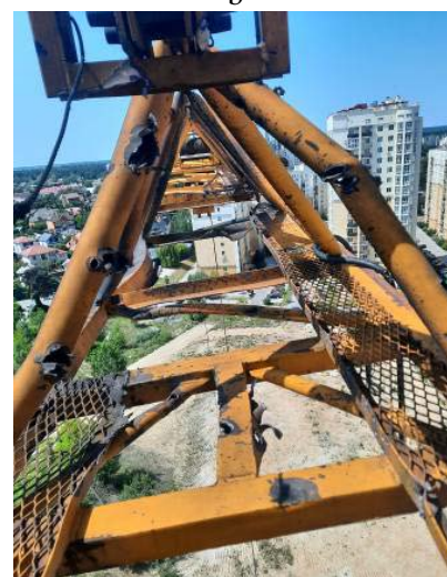
Fig. 3. Damage to metal structures from cannon shells: a – fastening of the cabin of the Simma Potain tower crane in Bucha; b – tower crane head KB403A, Irpin; c – boom section of tower crane FO23/B, Kyiv
