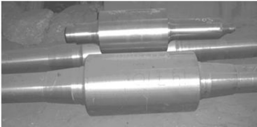
Fig. 2.6. Cast iron rolls manufactured by PJSC DZPV (Dnipro)
