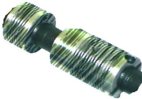
Fig. 3.6, a – Appearance goldsmith with became 38X2MUA after heat treatment and grinding
