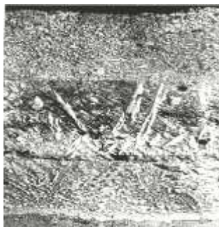
Fig. 12. General type of coating layer of PGSR +40% Cr 3 PRO 2 , ×400
