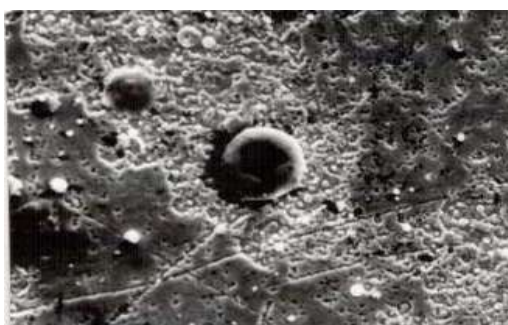
Fig. 11. Steel surface after bombardment with chromium ions, \times 1000
