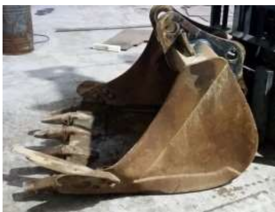
Fig. 2. Loss of shape of teeth of excavator buckets
