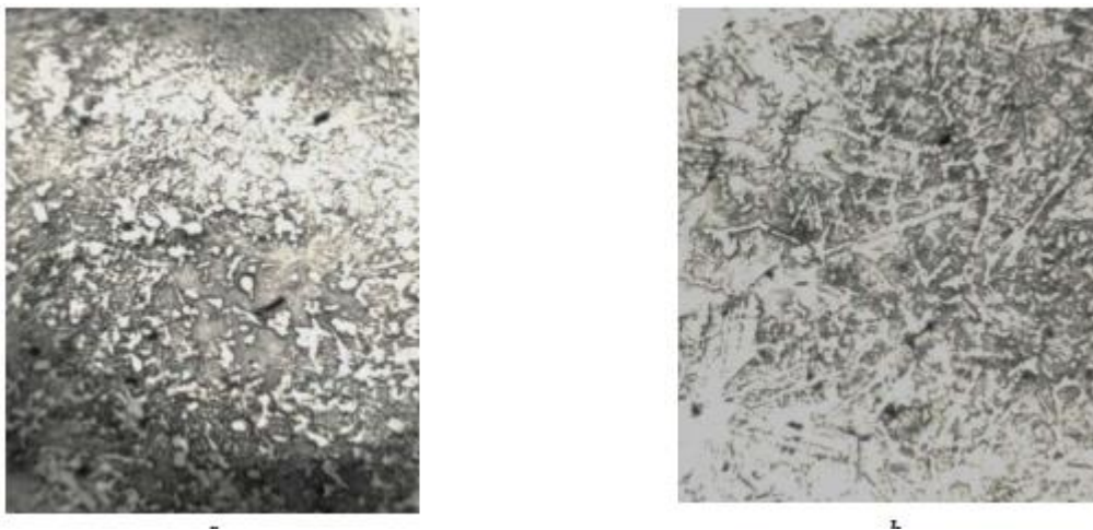
Fig. 2. Structure of powders for spraying PG-SR4 coatings
