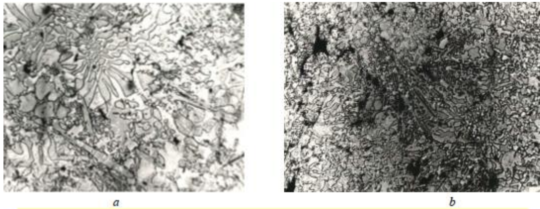
Fig. 6. The structure of the PG-SR4 molten coating layer: a – coarse mixtures; b – thin mixtures
