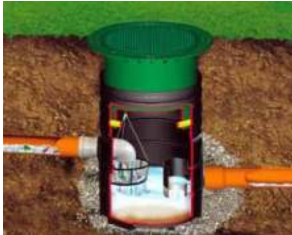
Figure 12.5 – Drainage inspection connection well
