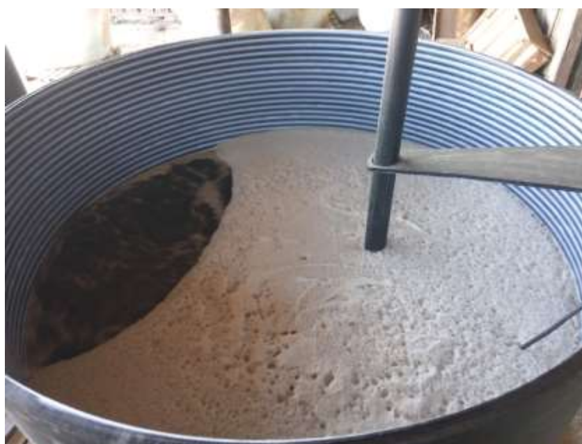
Fig. 8.1. Leachate aeration in the pilot-scale bioreactor tank
