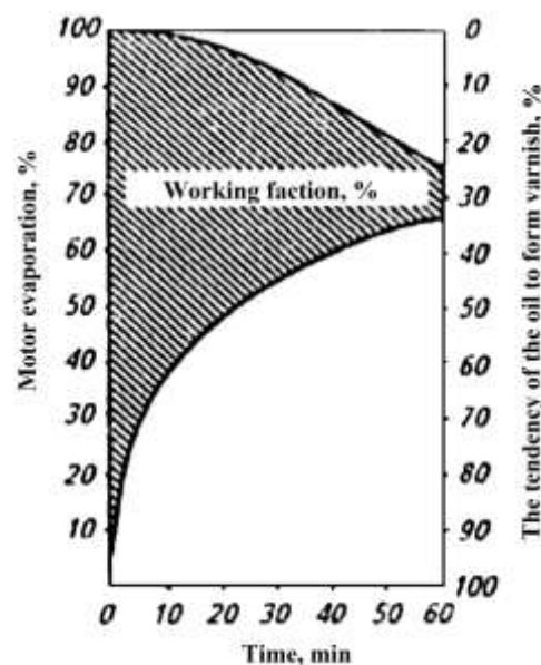
Figure 8.7 – Changes in motor evaporation, tendency to varnish and working fraction of motor oil at constant temperature
