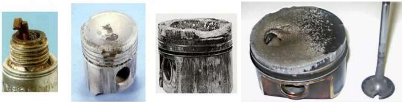
Figure 3.5 – Engine parts destroyed by detonation
