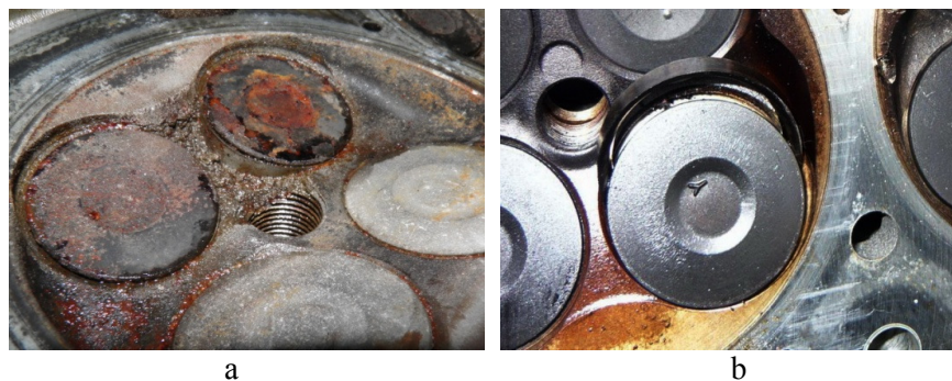
Fig. 9. Comparison of consequences of engines operating after loss of coolant: a – melting of the wall between the exhaust valves seats in the nominal mode of operation; b – and dropped valve seats of the cylinder head at idle speed operation
